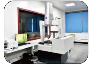
Zeiss Coordinate Measuring Machine(CMM)(Germany-made)
