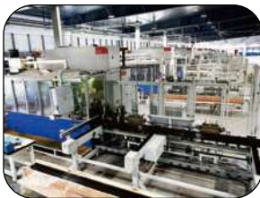
EFD Induction Hardening Equipment (Norway-made)
